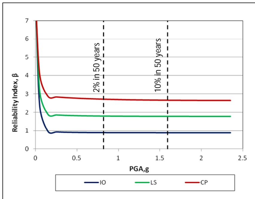
**Fig 4. Reliability Curves for 4S4B frame**
