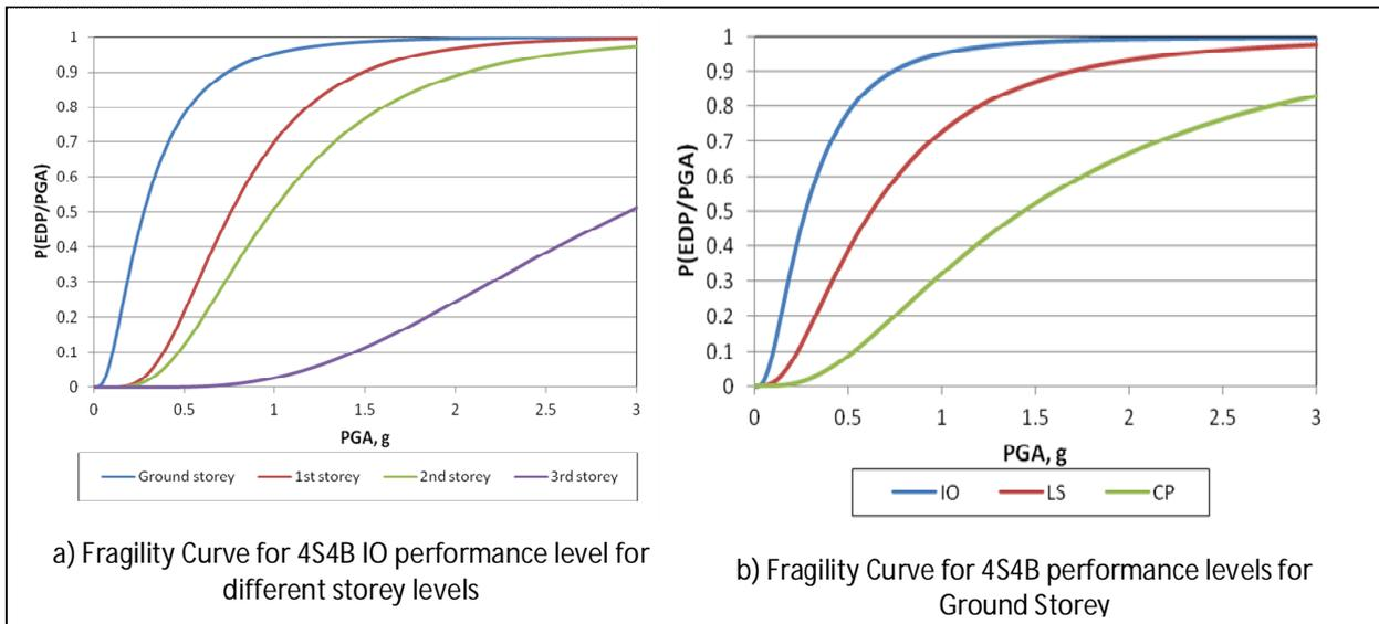
**Fig 3. Fragility Curves for 4S4B frame**
