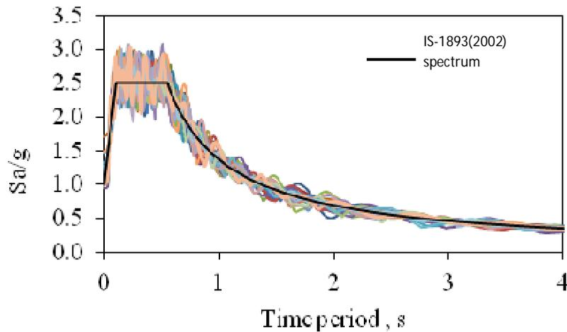
**Fig 2. Response Spectra for 44 converted ground motions along with IS 1893 (2002) design spectrum**
