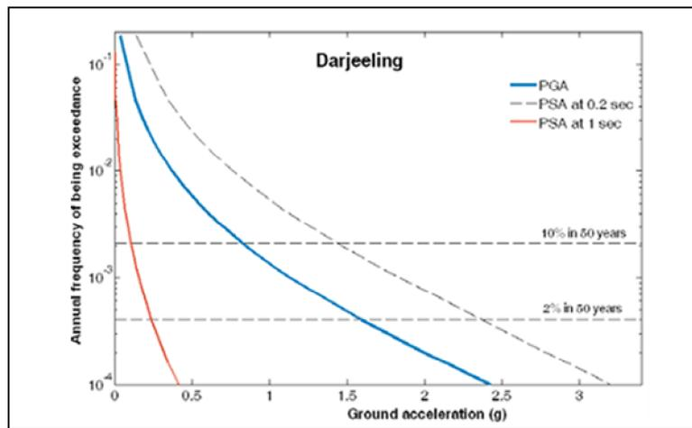
Fig 1 Seismic hazard curves of the Darjeeling region [4]
