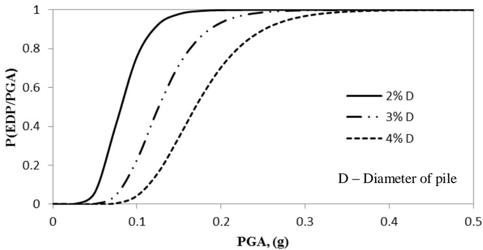
Figure 4 Fragility curves for design lateral deformation
