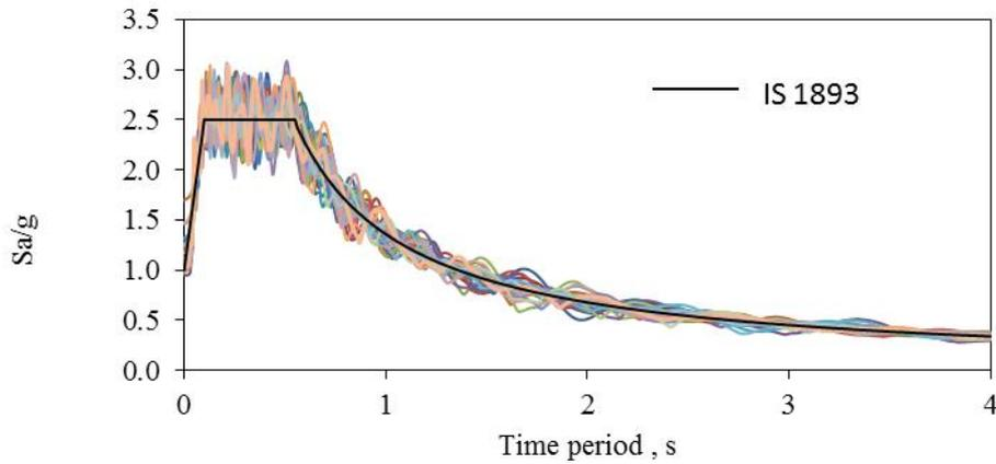
Figure 2 Response Spectra for 44 converted ground motions along with IS 1893 (2002) design spectrum axial strain curves
