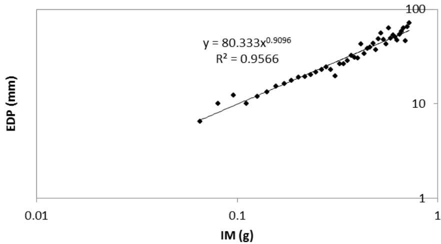
Figure 3 PSDM for Pile
