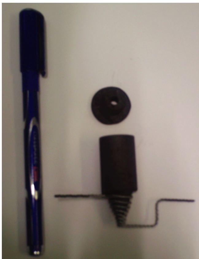
Figure 1. The arrangement of the filament with the graphite crucible.
