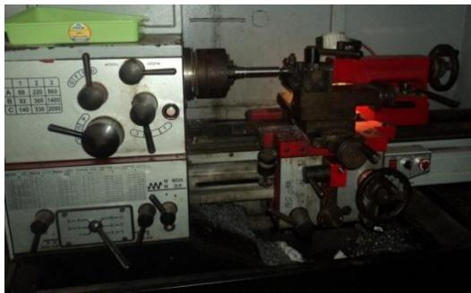
Fig.1 Photograph of experimental setup for turning of Inconel 825.
