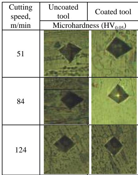
Fig.4 Optical microscopic images of Vickers indents on surface machined with different cutting speeds using uncoated and coated carbide inserts
