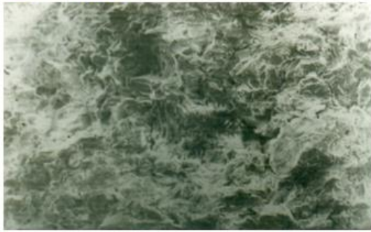
Fig. 1: YC+0%FA, TEMP 510°C, MGF 200X.
