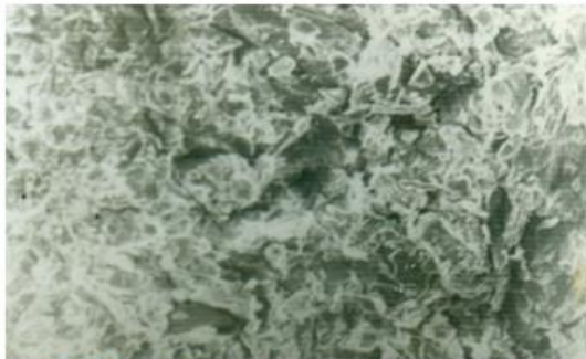
Fig. 3: YC+0%FA, TEMP 925°C, MGF 200X.
