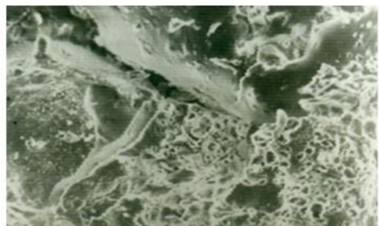
Fig. 8: BC+25%FA, TEMP 925°C, MGF 2000X.
