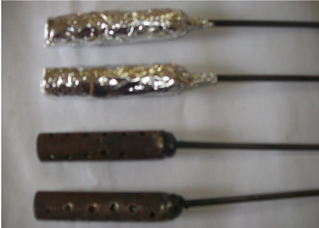
Fig. 2: Photograph of Perforated Mild Steel Capsule Welded to Plunger Rod (below), Mg or SiC Particles inside the Capsule Shown Wrapped with Al Foil (top).
