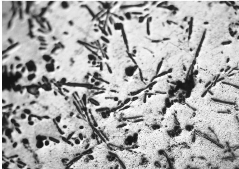
Fig. 6: Microstructure of Al-3 wt% Mg-10 wt% SiC MMC from the Bottom 10 mm of the Casting. Micrograph Shows Relatively Larger Size SiC Particles due to Gravity Sedimentation during Solidification of the Ingot.
