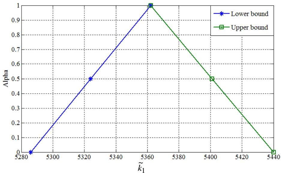
Figure 4. Identified lower and upper bounds of stiffness parameter  $\tilde{k}_1$  (N/m)
