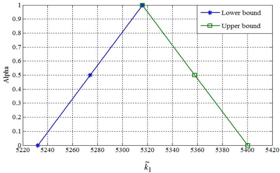
Figure 2. Identified lower and upper bounds of stiffness parameter  $\tilde{k}_1$  (N/m)
