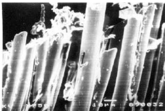
Figure 13 : Loss of adhesion between the fiber and the matrix
