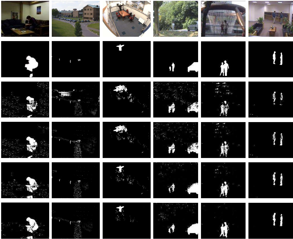
Figure 2: Left to right. Time of Day, PETS2001, Intelligent Room, Campus, Fountain, and Lobby frame sequence. Top to bottom. Original frame, Ground truth, and results of GMM, EGMM, Readdy et. al. , and LIBS.
