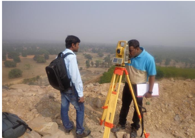
Fig 5: Total station for measuring Reduced Levels of monitoring stations
