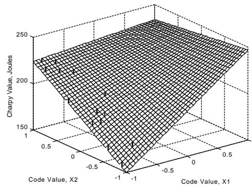
Fig. 12 - Charpy response surface (Region: 600 °C - 700 °C and 0.33 - 2 hours).
