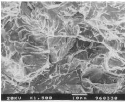
Fig. 7 - Fractograph of broken Charpy specimen (Quenched and tempered at 450 °C, 1 hour) shows quasicleavage nature.
