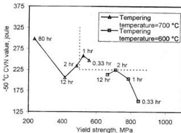
Fig. 9 - Yield stress vs. CVN value at different tempering temperature-time combinations.
