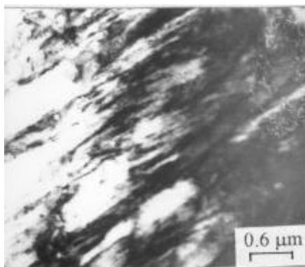
Fig. 4 - TEM of Quenched and tempered steel (600 °C, 1 hour) showing recovered structure.
