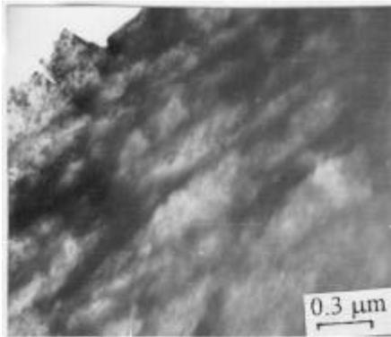
Fig. 3a - TEM of Quenched and tempered steel (450 °C, 1 hour) showing lath structure with dislocations.
