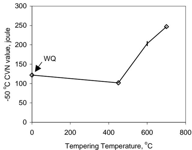
Fig. 6 - Variation of –50 °C CVN values with tempering temperature.
