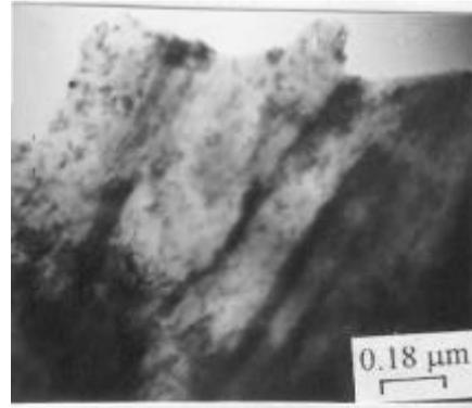
Fig. 3b - TEM of Quenched and tempered steel (450 °C, 1 hour) showing occurrence of precipitates due to tempering.
