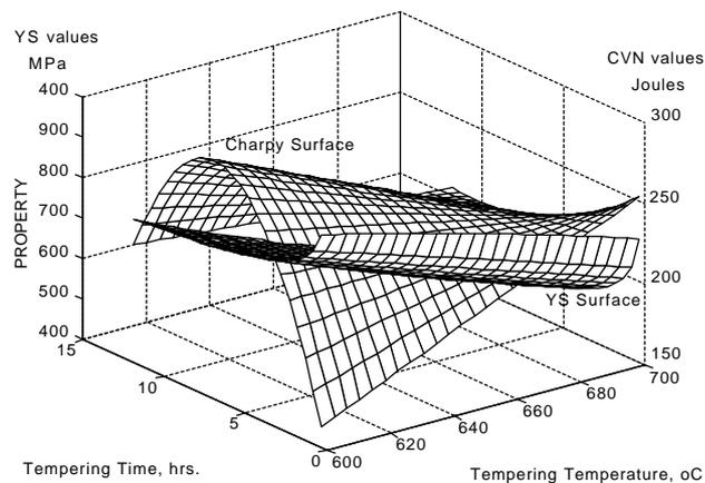
Fig. 11 - Yield strength response surface superimposed on Charpy response surface (Region:  $600^{\circ}\text{C}$  -  $700^{\circ}\text{C}$  and  $0.33$  -  $12$  hours).
