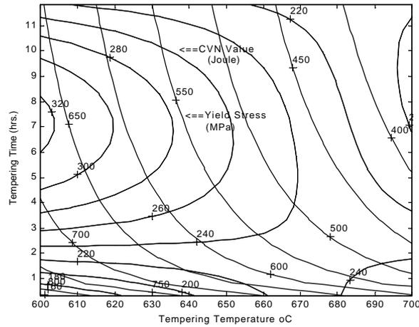
Fig. 10 - Contour plot of YS and  $-50^{\circ}\text{C}$  CVN value (Region:  $600^{\circ}\text{C}$  -  $700^{\circ}\text{C}$  and  $0.33$  -  $12$  hours).
