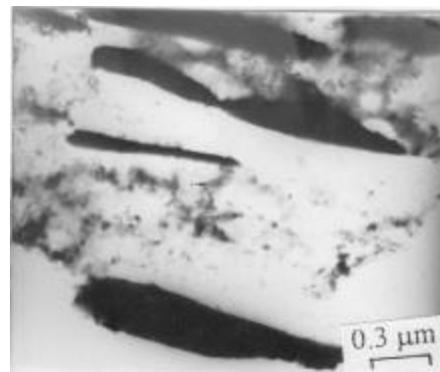
Fig. 5 - TEM of Quenched and tempered steel (700 °C, 1 hour) showing second generation austenite (dark regions) at lath boundaries.
