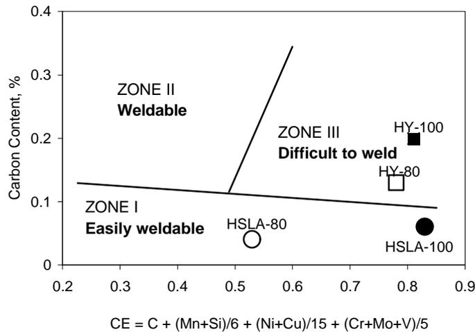
Fig. 1 - Relative positions of HY and HSLA steels in weldability diagram [4,5].
