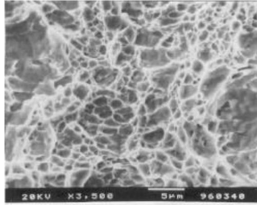
Fig. 8 - Fractograph of broken Charpy specimen (Quenched and tempered at 700 °C, 1 hour) shows dimple fracture.
