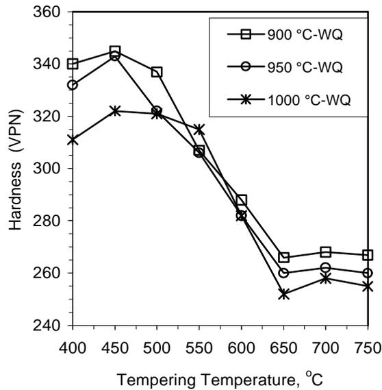
Fig. 2 - Tempering temperature vs. hardness curves.
