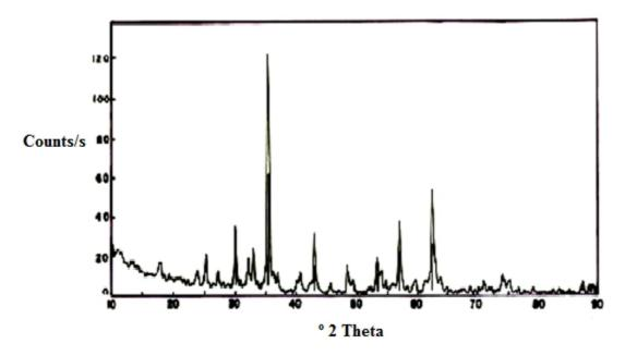
Fig. 8. X-Ray diffractogram of red mud coating deposited at 6 kW Operating power level
