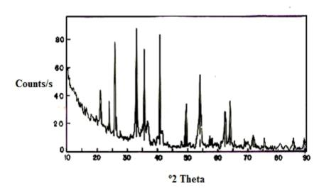
Fig. 7. X-ray diffractogram of red mud collected from NALCO
