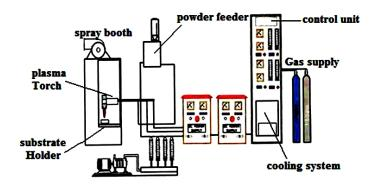
Fig. 1. Arrangement of the plasma spraying equipment
