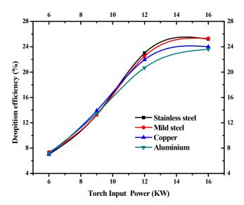
Fig. 10. Deposition efficiency of red mud coatings made at different power level at different substrates
