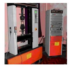
Fig. 2. Adhesion test set up Instron 1195
