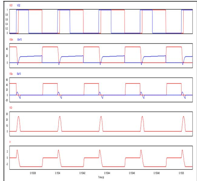
Fig. 8. Simulation waveforms : (a) Gating Signals ,(b) Voltage and Current across main switch ,(c) Voltage and Current across auxiliary switch, (d) Voltage across resonant Capacitor and (e) Current through resonant inductor  $L_r$
