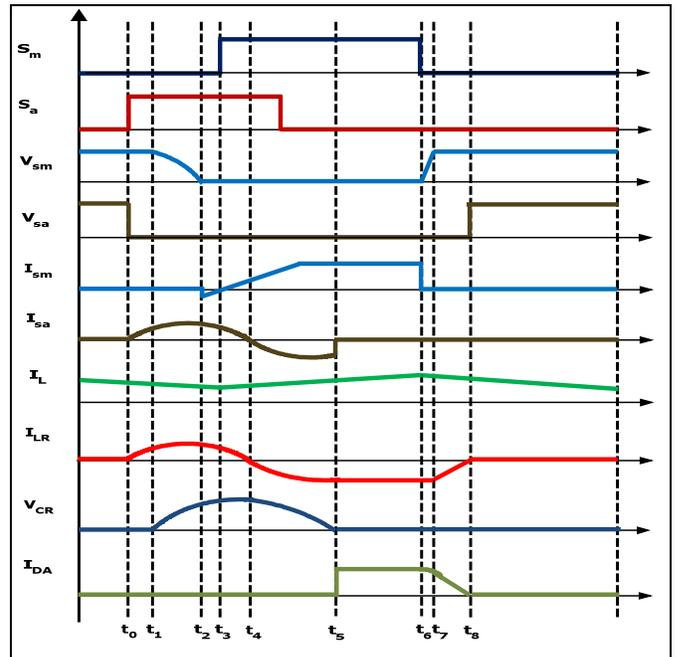
Fig. 5. Waveforms of the soft switching converter using an auxiliary resonant circuit
