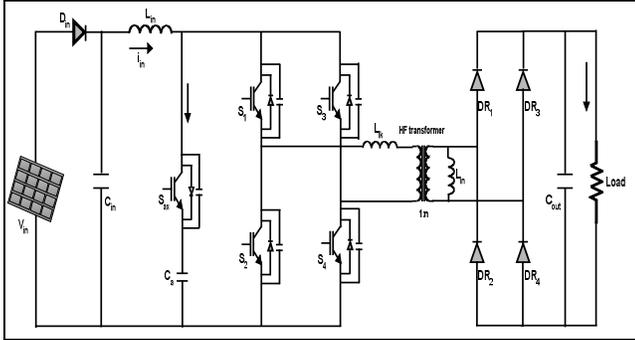
Fig.1. Active Clamped Current Fed Full-Bridge Isolated boost converter
