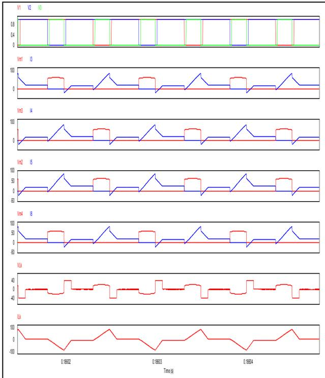
Fig. 7. Simulation waveforms : (a) Gating Signals to main switch and auxiliary switch ,(b) Voltage and Current through main switch  $S_1$  , (c) Voltage and Current through main switch  $S_2$ , (d) Voltage and Current through main switch  $S_3$ , (e) Voltage and Current through main switch  $S_4$ , (f) Voltage and Current through auxiliary switch  $S_{ax}$ , (g) transformer Volatge  $V_{AB}$  and (h) Leakage Inductor Current  $I_{L,K}$
