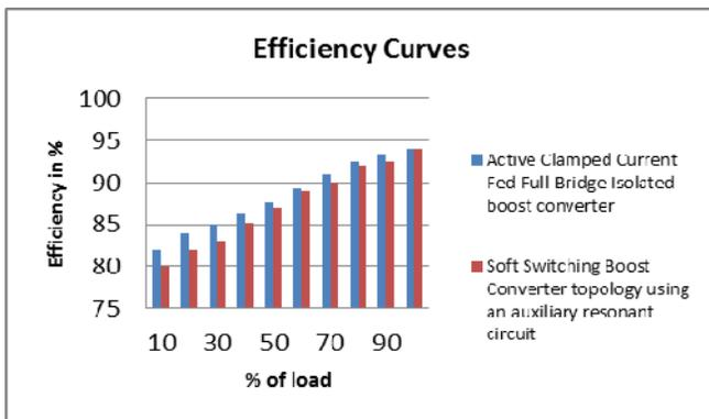
Fig.9. Variation in efficiency of the converters with changes in the percentage of load applied
