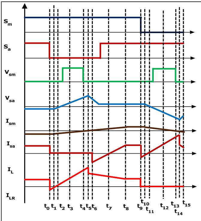
Fig. 3. Waveforms for the Active Clamped Current Fed Full-Bridge Isolated boost converter
