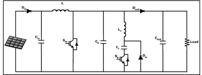
Fig. 4. Soft Switching Boost Converter topology using an auxiliary resonant circuit
