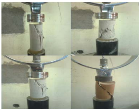
Figure 8: Failure of a few UCS samples
