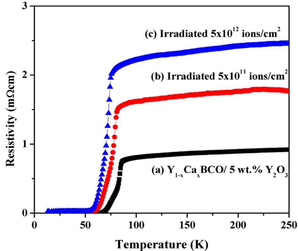
The ratio of  $\rho_{250K}/\rho_{100K}$  is  $\sim 1$  indicating that the fall of resistance is decelerated.
