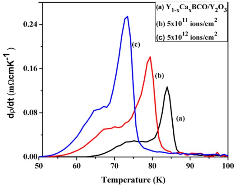
A finite tailing is observed in the derivative plot
