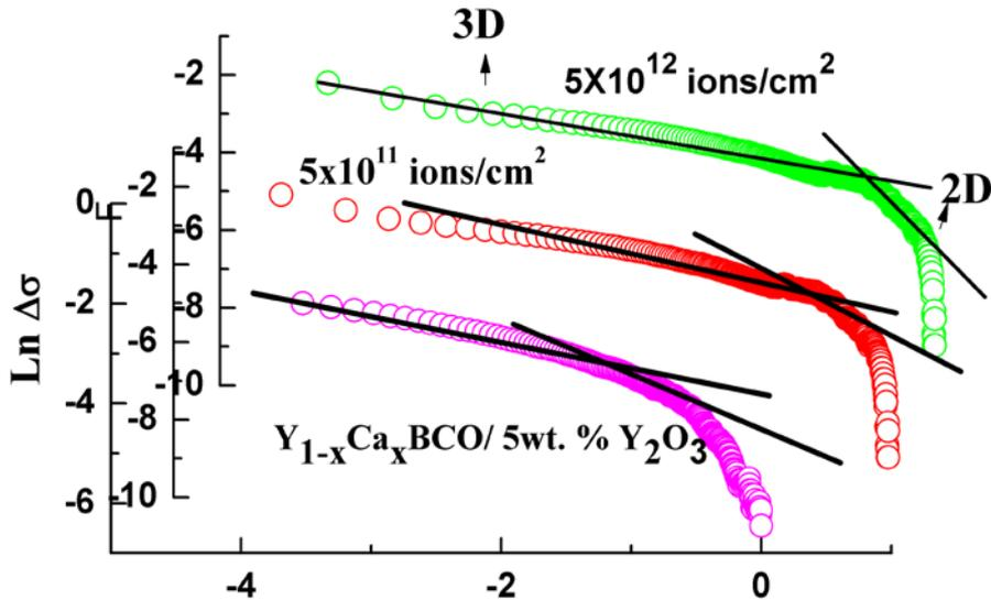
$T_{LD}$ ,  $T_{SWF}$  changes and 2D regime dominates the flow of activated charge carriers in irradiated samples.
