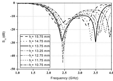
Fig. 3 Comparison of S parameters at various height of the triangular DR
