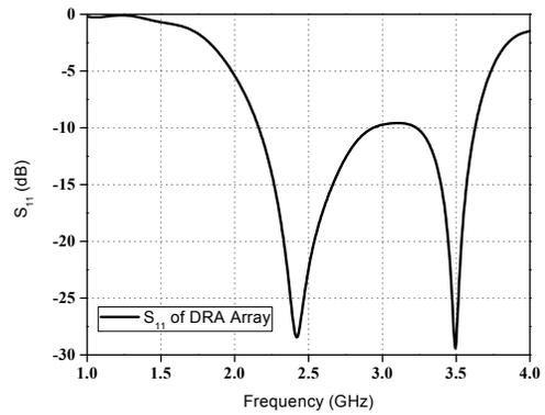
Fig. 4 S parameter of proposed triangular DRA array
