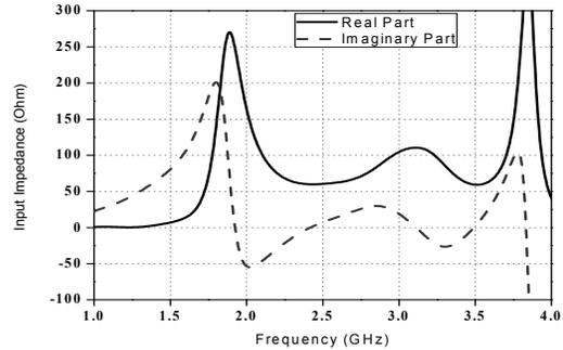
Fig. 6: Input Impedance for Triangular DRA array
