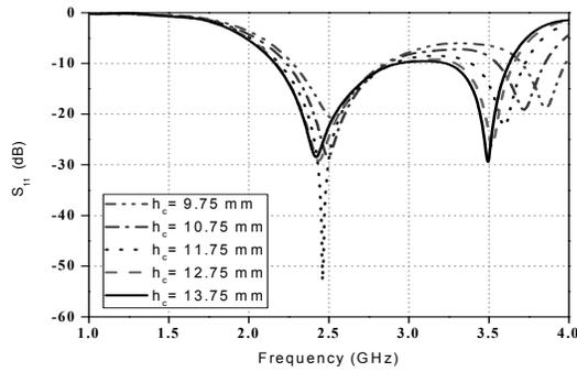
Fig. 2 Comparison of S parameters at various height of the conformal patch
