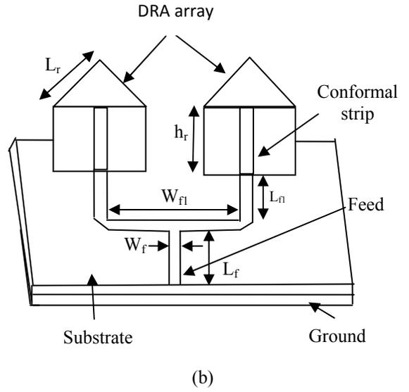
Fig. 1 (a) Geometry and (b) Schematic view of the Triangular shaped Dielectric Resonator Array
