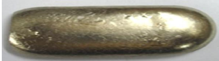
Fig: 2 Prepared sample of NiMnSn Heusler FSMA
