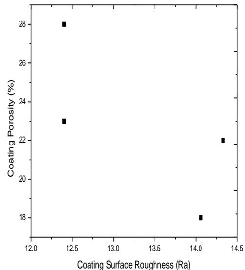
**Fig. 6:** Variation Coating Surface Roughness with Coating Porosity for Copper Substrate.
