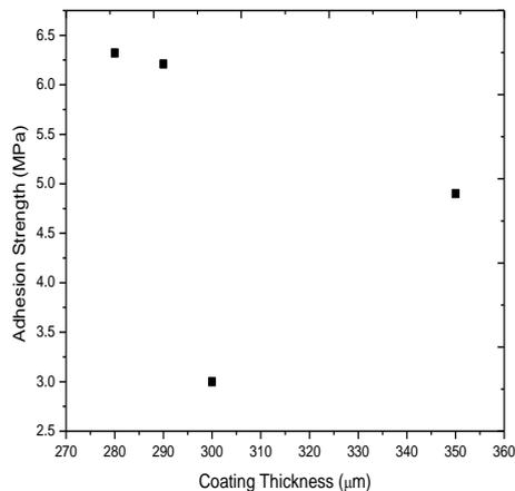
**Fig. 3:** (b) Variation of Adhesion Strength with Coating Thickness (Copper).
