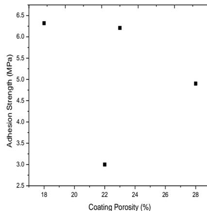
**Fig. 4:** Variation of Adhesion Strength with Coating Porosity for Copper Substrate.
