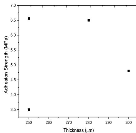
**Fig. 3:** (a) Variation of Adhesion Strength with Coating Thickness (Mild Steel).
