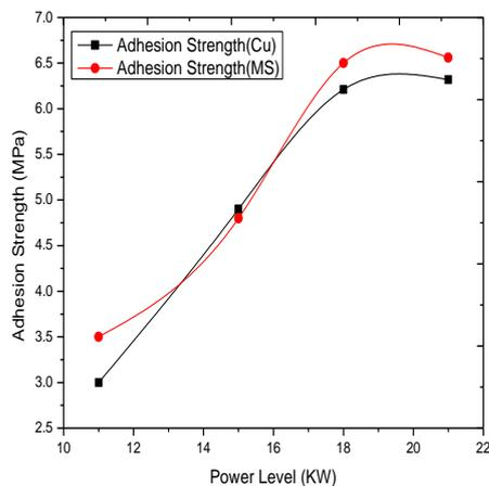
**Fig. 2:** Comparison of Adhesion Strength of Mild Steel and Copper with Respect to Power Level.
