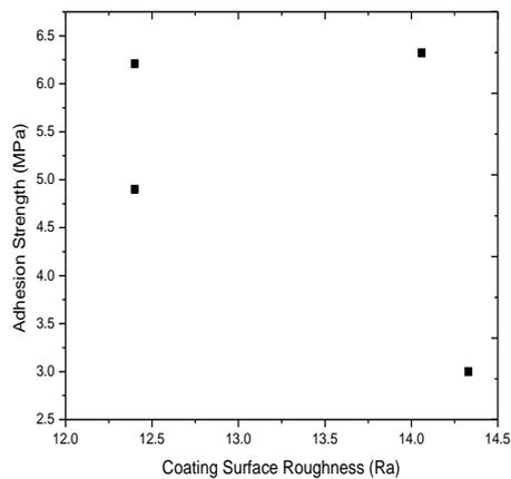
**Fig. 5:** Variation of Adhesion Strength with Coating Surface Roughness for Copper Substrate.
