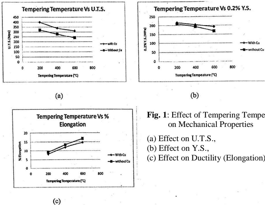
**Fig. 1:** Effect of Tempering Temperature on Mechanical Properties
