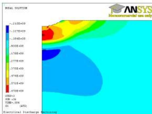
Figure 3 Radial component of residual stress ( $\sigma_{rr}$ ) at the end of pulse period.
