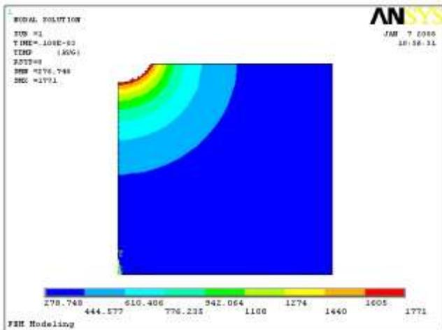
Figure 2 Temperature profile of workpiece after metal vaporization
