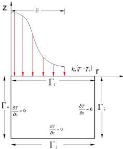
Figure 1 Axisymmetric thermal model
