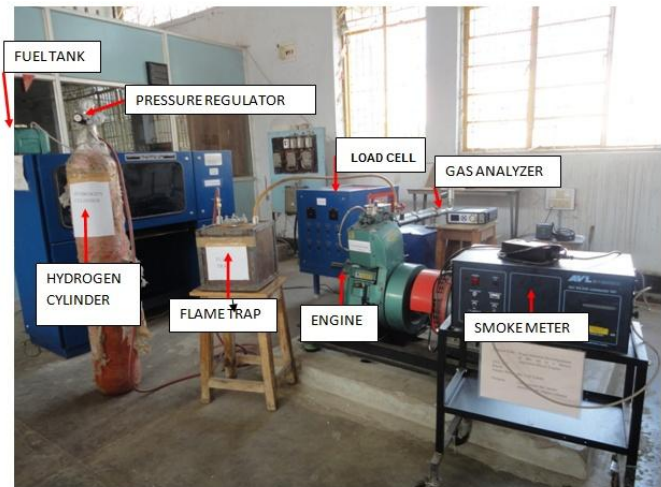
Fig.1 Photographic representation of the engine experimental set up
