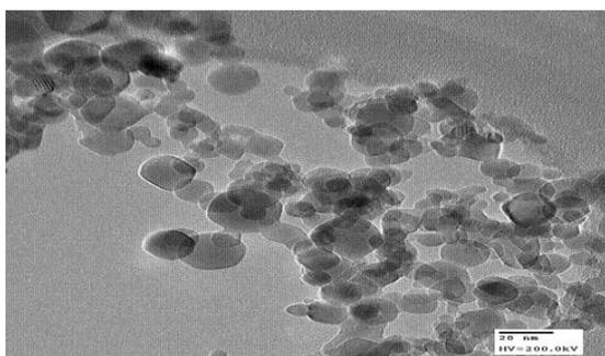
**FIGURE 2.** TEM photographs of reactive plasma synthesized nanocrystalline  $ZrO_2$
