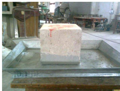
Fig. 2. Capillary absorption test of cubes.
