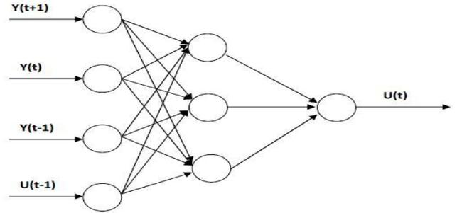
Fig.1 DINN network architecture in control mode.
