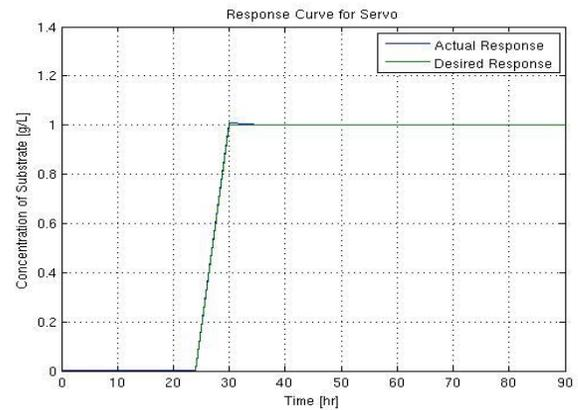
Fig.4 Response in substrate concentration for unit step change in dilution rate using conventional servo nutristat controller (trained network with 2 time unit sampling interval).
