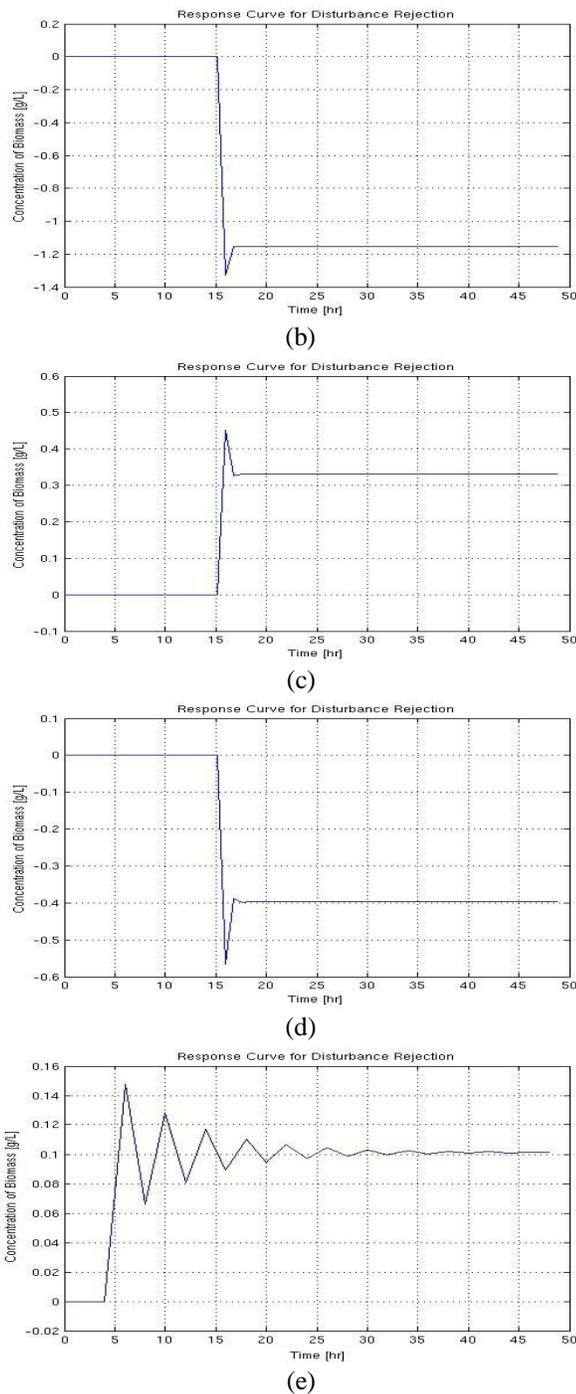
Fig.5 Disturbance rejection by concentration turbidostat: in (a) in  $\mu_{max}$  (b) in  $k_m$  (c) in  $Y$  (d) in  $D$  (e) in  $x_{2f}$
