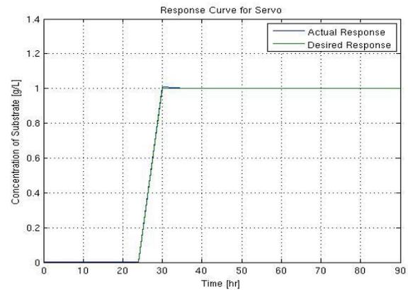
Fig.4 Response in substrate concentration for unit step change in dilution rate using conventional servo nutrstat controller (trained network with 2 time unit sampling interval).
