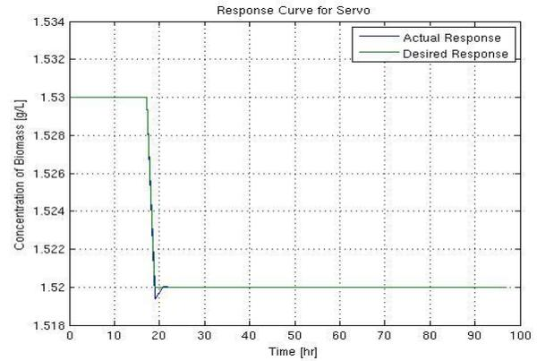
Fig.3 Response in biomass concentration for unit step change in dilution rate using conventional servo turbidostat controller (trained network with 0.8 time unit sampling intervals).
