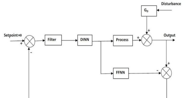
Fig.2 Block diagram of closed loop IMC scheme.
