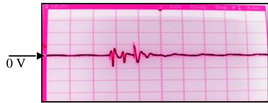
Fig.10. Voltage could not build up and collapses for a prime mover speed of 1090 rpm
