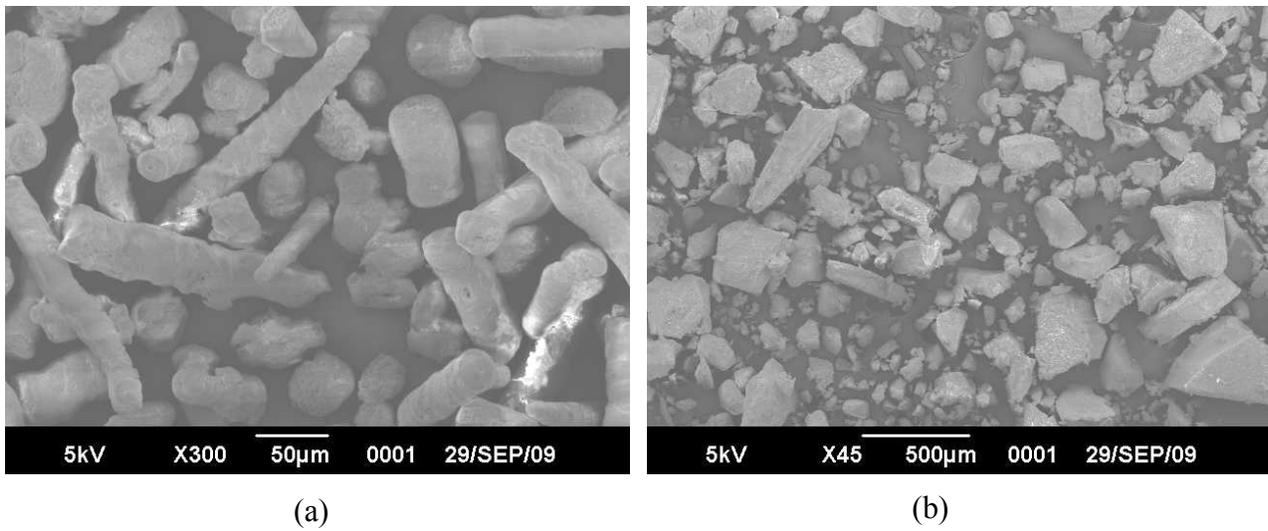
Figure 4. Scanning electron micrographs of (a) HPMC and (b) HPMCAA
