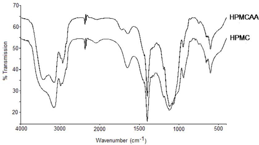
Figure 1. FTIR spectra of HPMC and HPMCAA
