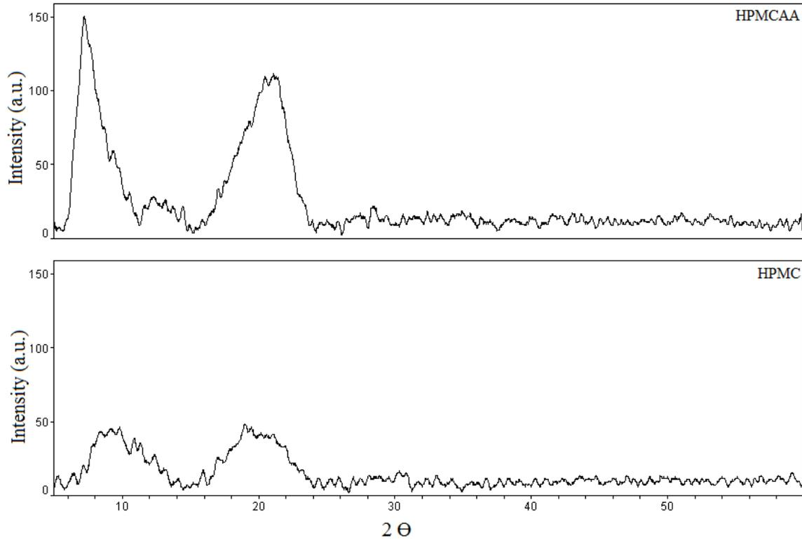
Figure 3. XRD profile of HPMC and HPMCAA
