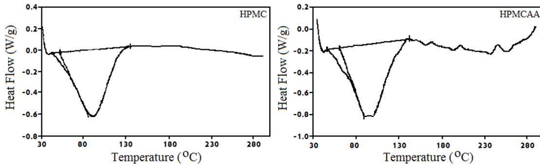
Figure 2. DSC thermogram of HPMC and HPMCAA
