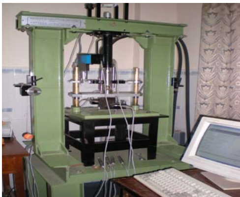
Fig. 1 Repeated load indirect tensile test setup
