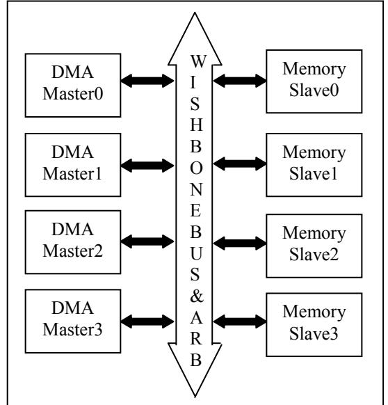
Fig. 2 Proposed Shared Bus System Architecture
