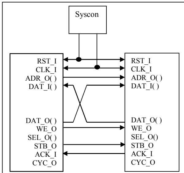
Fig. 1 Proposed Point-to-Point System Architecture
