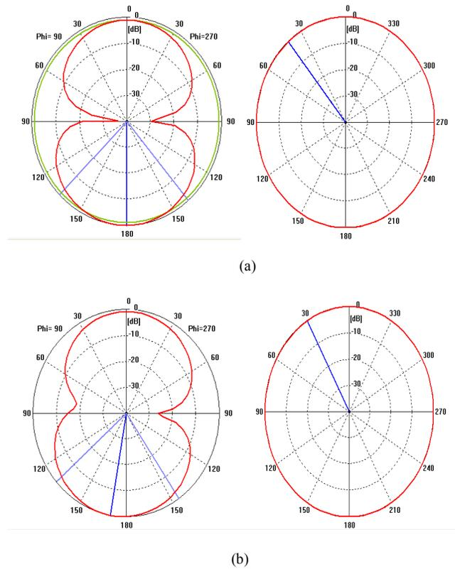
Fig. 6 Simulated E plane (left) and H plane (right) radiation patterns of Ring DRA at (a) 3.9 GHz and (b) 6.5 GHz
