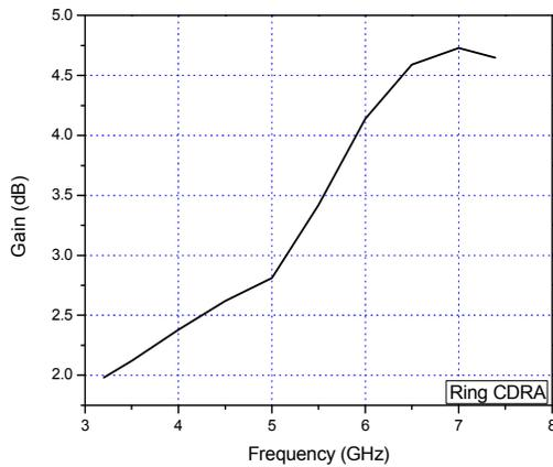
Fig. 4 Simulated Gain of the Ring DRA versus Frequency
