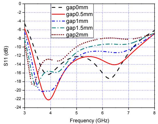
Fig. 3 Simulated return loss with different values of air gap
