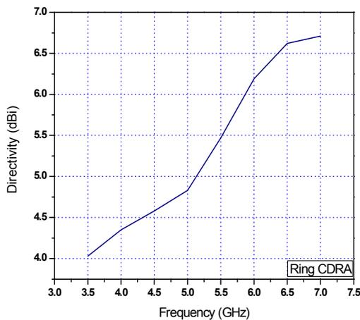
Fig. 5 Simulated Directivity versus Frequency
