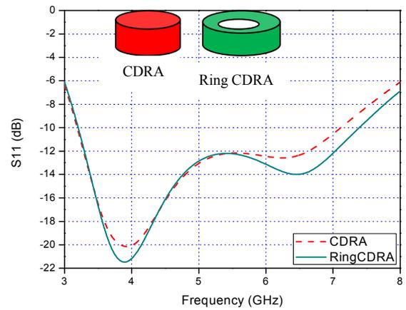
Fig. 2. Comparison of return loss plot of a typical cylindrical DRA (CDRA) with a ring DRA (Ring CDRA).
