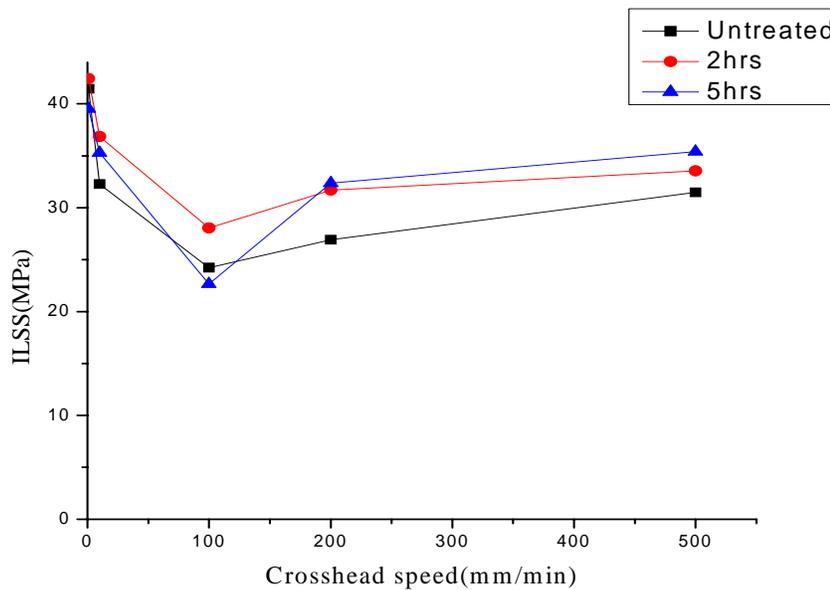
Fig.3 (a) Crosshead speed Vs ILSS for carbon/epoxy composites above ambient temperature at + 50°C for 2 and 5 hours conditioning time
