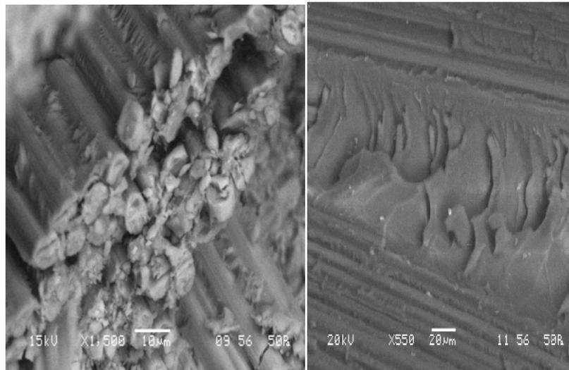
Fig.4. (a) Showing matrix cracking, fiber/matrix de-bonding, fiber fracture and fiber pullout at higher cross head speed and fig4.(b) depicts developments of cusp due to shear stress in CFRP.
