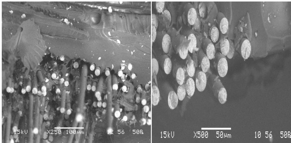
Fig.2(a) Showing extensive fiber/matrix de-bonding and fiber pullout in glass/epoxy composite at higher cross head speed and fig. 2(b) depicts increase fiber/matrix adhesion due to thermal conditioning.
