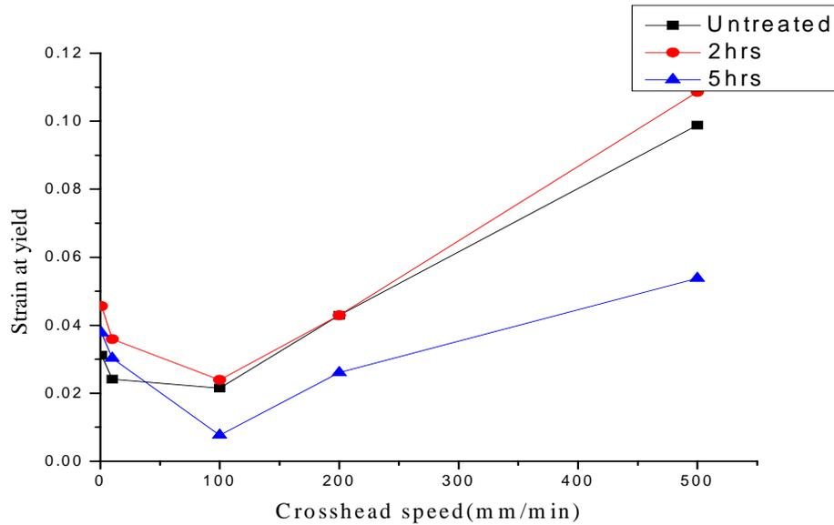
Fig.3(b) Strain at yield Vs Crosshead speeds of carbon/epoxy composites above ambient temperatures at + 50°C for 2 and 5 hours conditioning time
