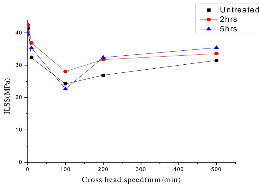
Fig.1 (a) Crosshead speed Vs ILSS for carbon/epoxy composites above ambient temperature at + 50°C for 2 and 5 hours conditioning time.
