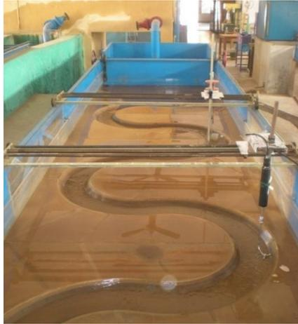
**Photo 1: Type-IV Experimental channel with measuring equipments.**
