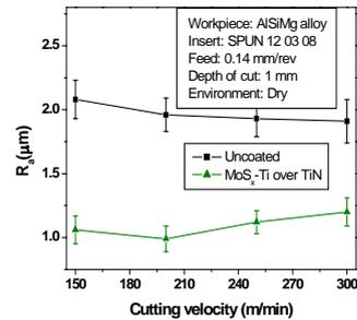
**Fig 4.** Variation of workpiece surface roughness (R<sub>a</sub>) with cutting velocity during dry turning of aluminium alloy with uncoated and coated inserts
