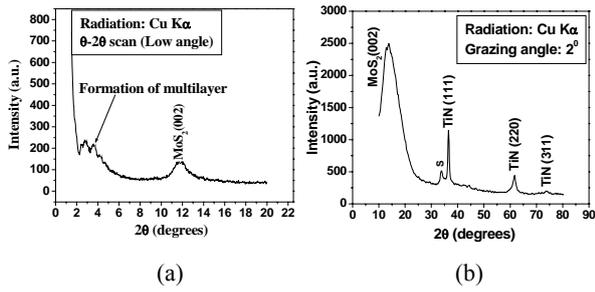
**Fig 2.** (a) Low angle XRD and (b) GIXRD spectra of MoS<sub>x</sub>-Ti coating with TiN underlayer
