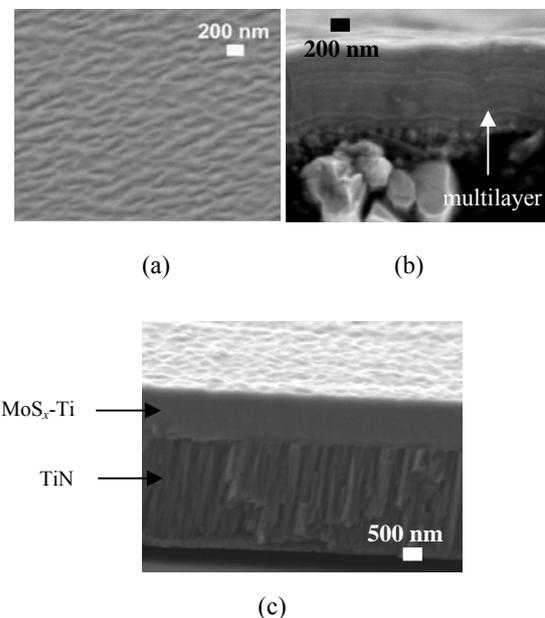
**Fig 1.** SEM micrographs of showing (a) surface morphology, (b) fractograph of MoS<sub>x</sub>-Ti coating and (c) fractographs of MoS<sub>x</sub>-Ti with TiN underlayer
