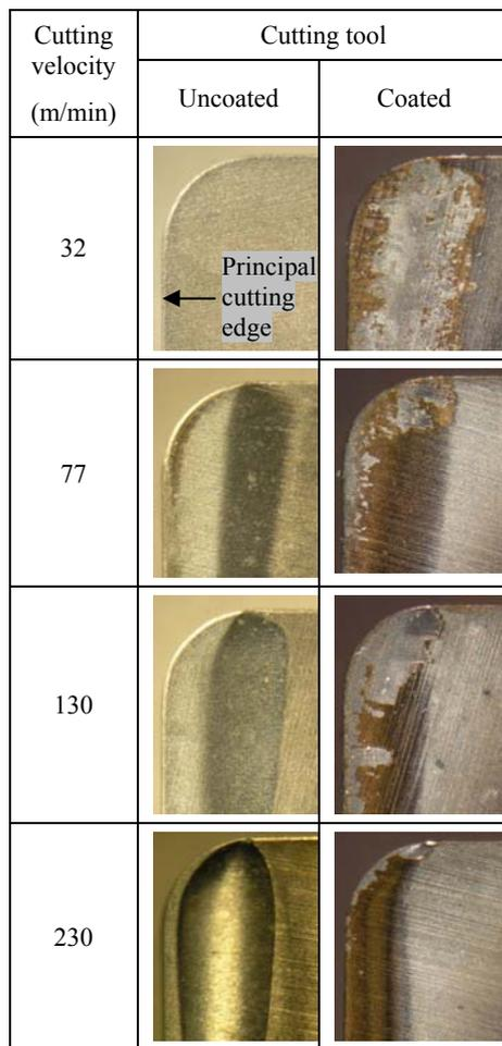
**Fig 6.** Optical microscopic images showing rake surfaces of uncoated and coated turning inserts after machining of steel with different cutting velocities
