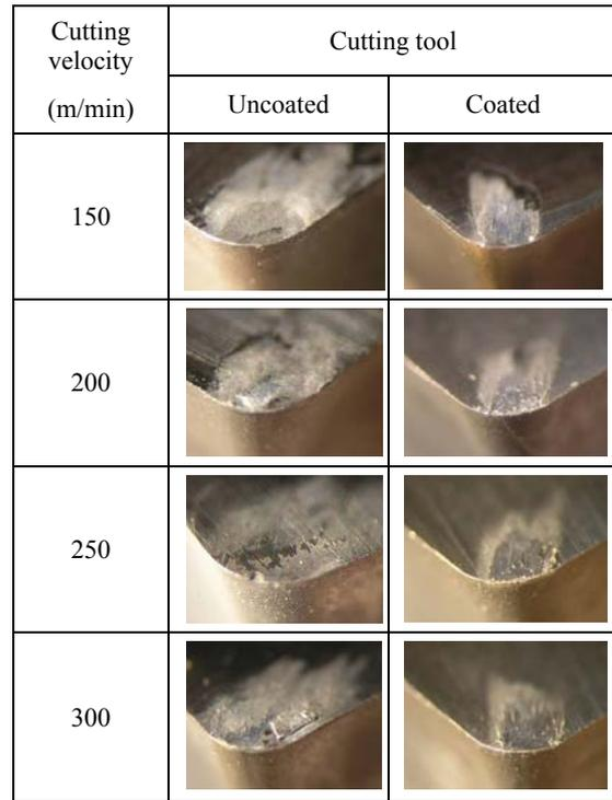
**Fig 3.** Optical micrographs of uncoated and coated turning inserts after machining of aluminium alloy with different cutting velocities
