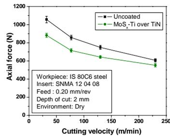
**Fig 5.** Variation of axial cutting force (P<sub>x</sub>) with cutting velocity during dry turning of steel with uncoated and coated inserts
