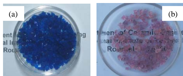
Figure 1. (a) dried blue silica gel and (b) humidified blue silica gel
