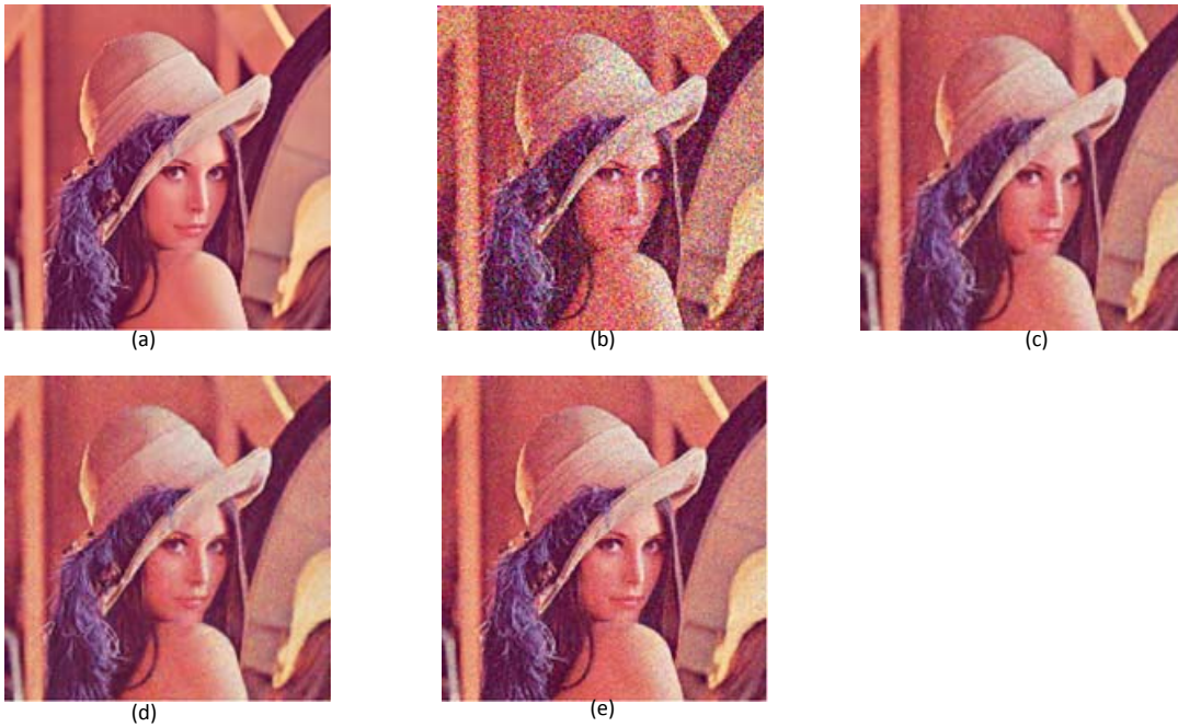
Figure 4. Performance of Various Filters in YCbCr-Color Space for Color Lena Image with AWGN of \sigma_n = 40 (a) Original image (b) Noisy image (c) – (e): Results of various filtering schemes (c) M-MF (d) M-LAWML (e) Proposed Filter: MCSF
