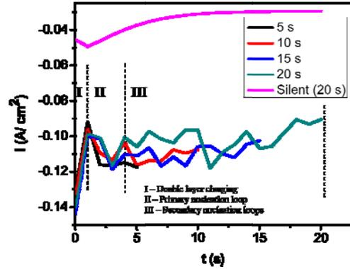
Fig.1. Chronoamperometric current transients for Cu deposits under insonation for different time periods
