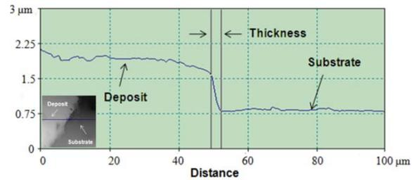
Fig. 2: AFM micrograph of sonicated deposit at 20 s (Thickness measurement)
