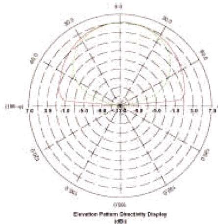
Figure 7 Radiation pattern of dual-fed Balanced Amplifying Antenna (Red line  $E_0$  and green line  $E_90$ )
