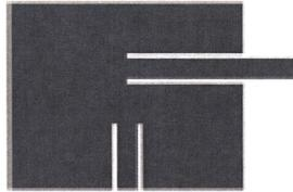
Figure 3 Orthogonal Dual Fed Patch Antennas
