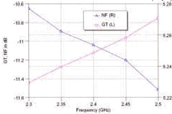
Figure 6 Gain and Noise Figure of the Dual Fed Balanced Amplifying Antenna
