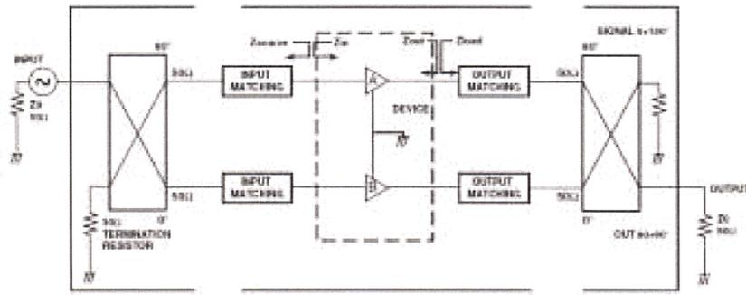
Figure 1 Schematic of Balanced Amplifier
