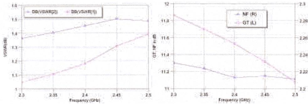
Figure 2 (a) VSWR at the input (#1) and output (#2) ports. (b) Response of Balanced Amplifier
