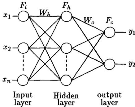
Fig. 1. Schematic diagram of a Multilayer Feedforward Network
