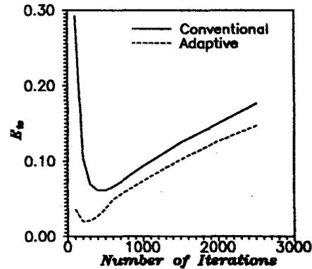
Fig. 3. Variation of MSSE of the test data as a function of the Number of iterations for Conventional and Adaptive BPA
