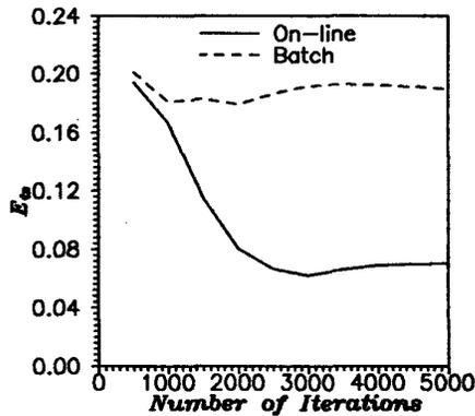
Fig. 2. Variation of Mean sum squared error as a function of iterations for On-line and Batch procedure of learning (Model -III)
