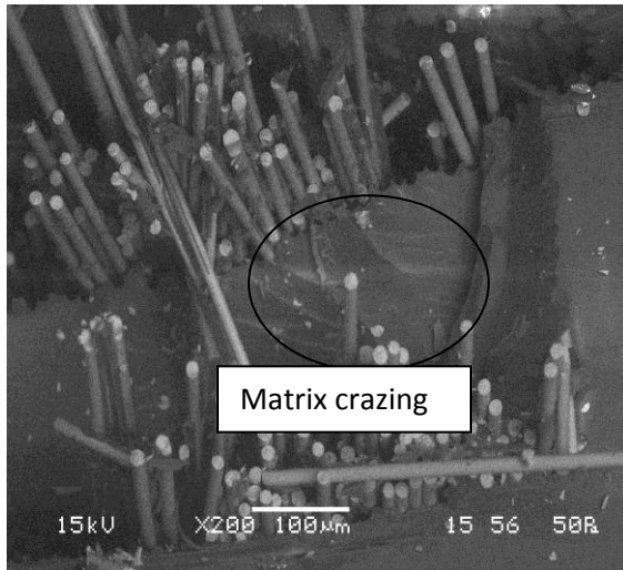
Fig.6 Matrix damage is leading to matrix crazing in glass-epoxy composite.
