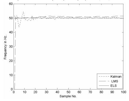
Estimation of frequency by different algorithms is superimposed in Figure 5 with SNR of 30 dB. From Figure 5, it is clear that KF approach exhibits more oscillation and does not settle around 50 Hz. At the same time, LMS approach exhibits oscillations in the few initial samples and finally settles around 50 Hz. But ELS algorithm exhibits fewer oscillations and also settles around 50 Hz. So the estimation of frequency by ELS algorithm is preferred.
