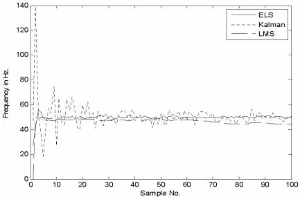
Figure 4 Comparison of estimation of power system frequency at SNR (20 dB)
