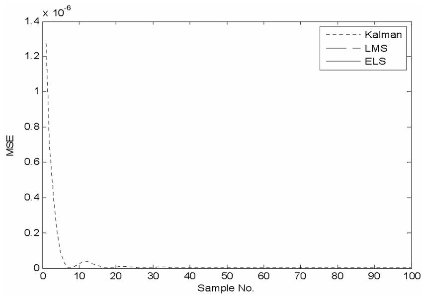
From Table 1, the computational time for estimation of frequency by ELS algorithm is 0.2340 seconds, which is less in comparison to other two methods. The estimation error (RMS) in the case of ELS algorithm is also less in comparison to other two methods.
